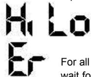
'Hi' or 'Lo' is displayed when the temperature being measured is outside of the range of the instrument. 'Hi' when higher than 428°F and 'Lo' when lower than -27°F in infrared mode and 626°F and -67°F respectively with the contact probe.
