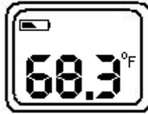
'Battery Low' : Battery needs to be replaced, measurements are possible
